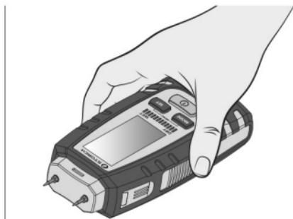
Always hold and press down the measuring device in the same way (see illustration).
