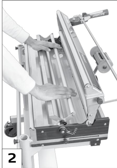
Insert the aqua adapter into the locking mechanism. The square strut is aligned with the table side of the Tapetomat.
