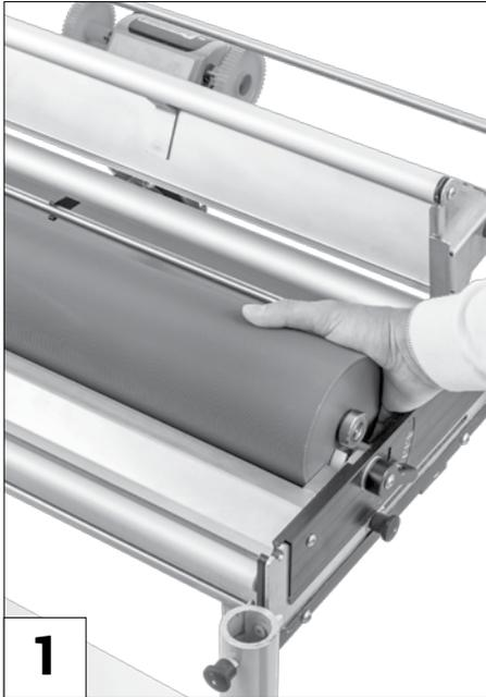
Before installing the aqua adapter, the standard wallpaper paste roller must be removed from the Tapetomat unit.
