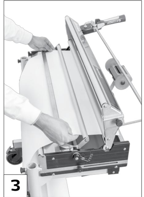
Insert the wall covering below the two top struts and push it forward until it sits on the wallpaper trays.
