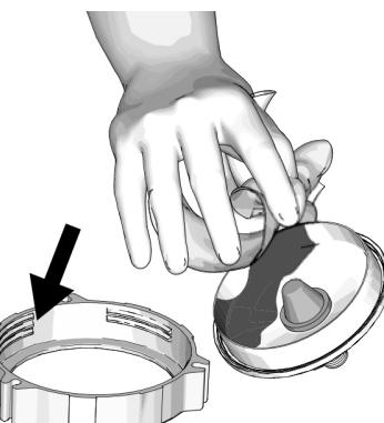
7. Fill the cupinlet (4) approximately half-full with cleaning fluid (warm water or appropriate solvent).
