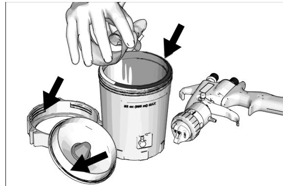
4. Install cover and ring onto cup. Tighten ring securely.
