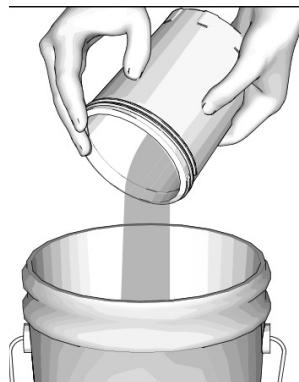
5. It is recommended to dispose of the used cupinlet (4) and install a new one. If reusing, clean by wiping all excess fluid from cupinlet (4).
